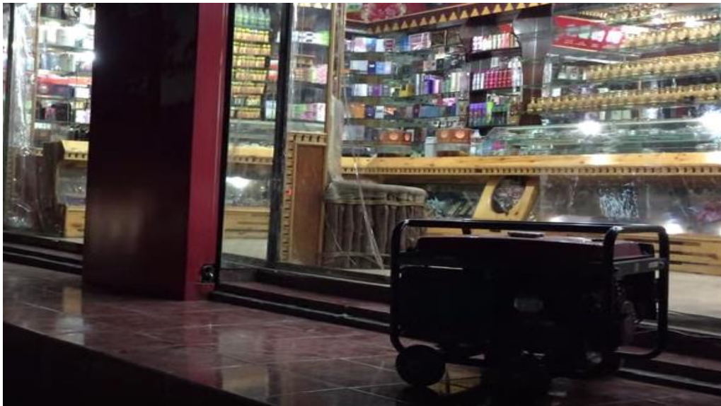
Figure 6: Businesses rely on gas-operated power generators like this one outside a shop. (Photo credit: Naser Noor)
